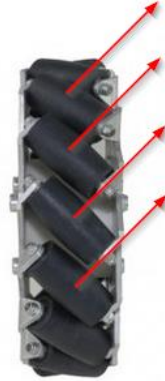
Figure 4.2.1-1 Mecanum Wheel Force Direction
