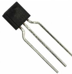
Figure 4.3.1-4 Example of the smaller package size of a typical BJT (Reprinted with permission from Sparkfun)
