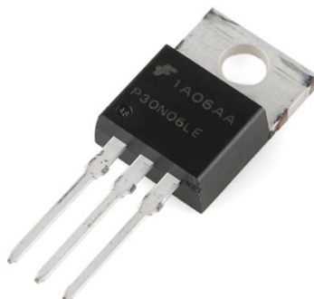
Figure 4.3.1-5 Example of the larger package of a FET (Reprinted with permission from Sparkfun)
